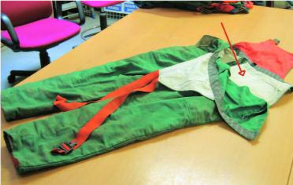
Tuta da motoseghista con imbottitura in fibre sintetiche (freccia rossa)/Chainsaw operator's overalls with synthetic fibre stuffing (red arrow)
